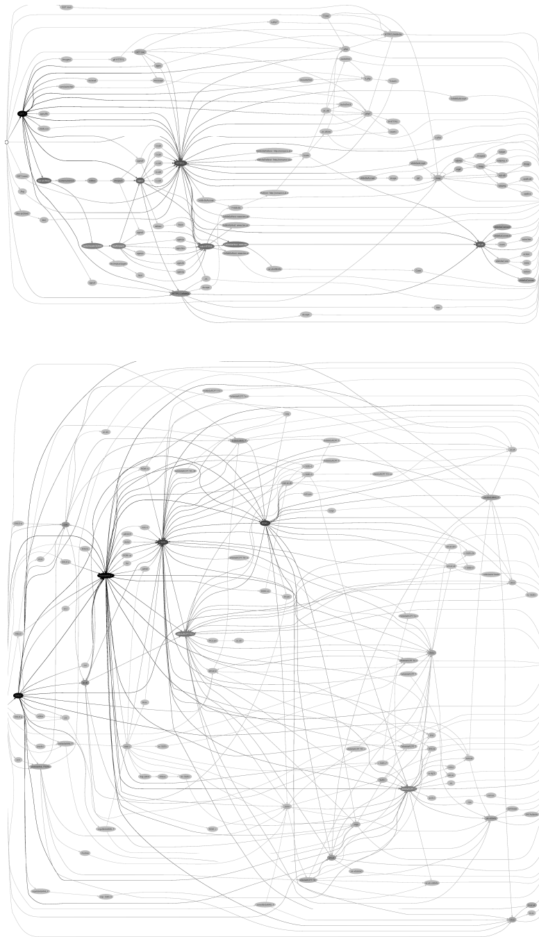
Figure 4.7. CSGs for TCP protocols HTTP (top) and SMTP (bottom), flow prefix length 100 bytes, soft node limit 100 nodes. Heavier nodes are rendered in a darker background. Observe that only a small number of nodes are heavy.
