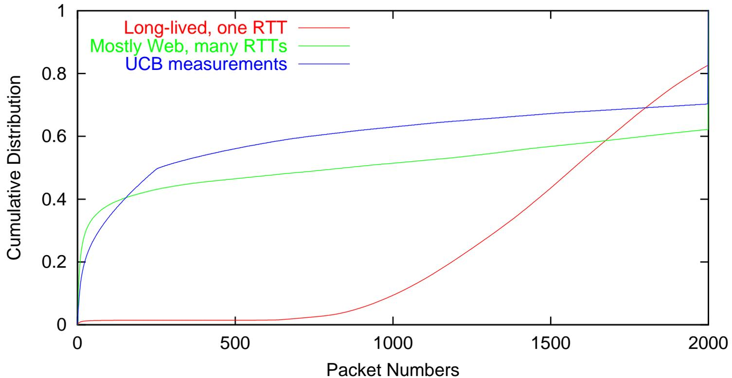
Distributions of packet numbers on the congested link over the second half of two simulations, with data measured on the Internet for comparison.
