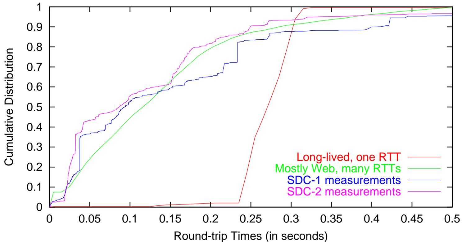
Distributions of packet round-trip times on the congested link of two simulations, with data measured on the Internet for comparison.
