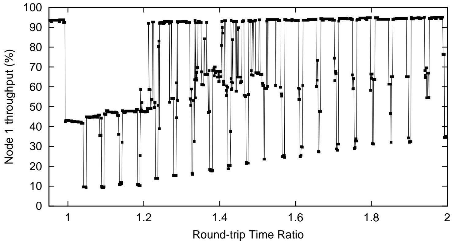
Flow 1's throughput as a function of the ratio of the two flows' round-trip times
