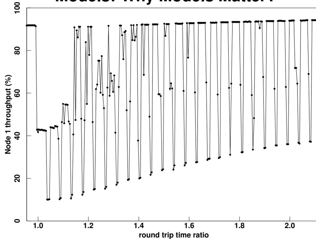
Flow 1's throughput as a function of the ratio of the two flows' round-trip times, in a scenario with one-way traffic and Drop-Tail queue management. [From "On Phase Effects", 1992.]
