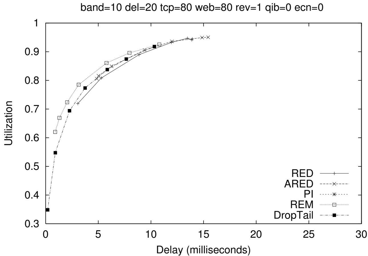
Steady-state simulations, with some web traffic and reverse-path traffic, and 40-320 ms RTTs. Queue in packets.
