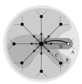
Fig. 3. Dispatching events to varying subsets of the subscriber set: the white node sends an event to the central node, whose processing triggers another event to which all of the ring nodes are subscribed. Depending on the central node's dispatching policy, different subsets of the subscriber set are included: (A) full broadcast, (B) limited broadcast, (C) subgroup, (D) sender only.
