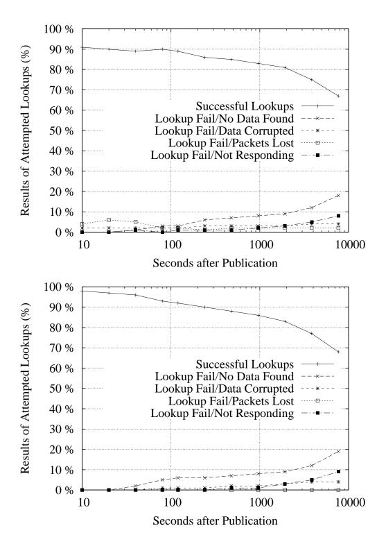
Figure 6.1: Bit pipe retrieval results for the TTL (top) and Recursion Desired methods.
