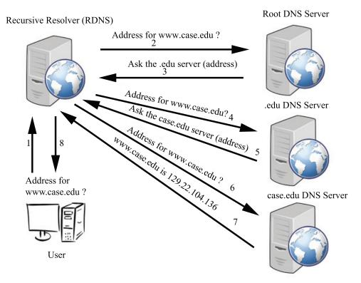
Figure 2.2: DNS Resolution Process
