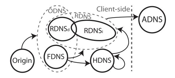
Figure 4.1: Structure of the client-side DNS infrastructure.
