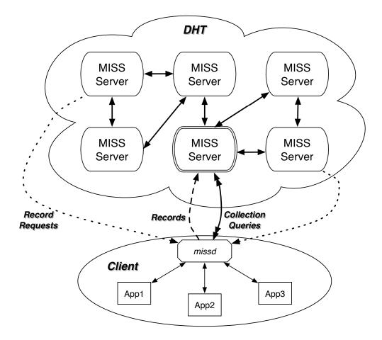
Figure 7.2: Conceptual diagram of MISS system.
