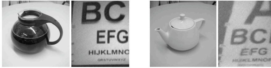
Figure 6. Reflections in two other tea pots, taken from a distance of 5m. The 18pt font is readable from the reflection in the left picture, and almost readable in the right picture.
