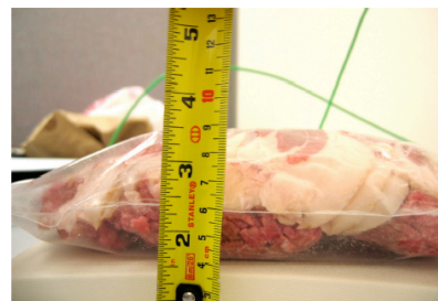
Fig. 8. To simulate implantation in a human, we placed the WISP in a bag containing bacon and ground beef.
