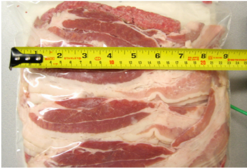
Fig. 8. To simulate implantation in a human, we placed the WISP in a bag containing bacon and ground beef.
