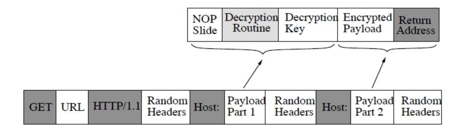
Figure 1. Polymorphed Apache-Knacker exploit. Unshaded content represents wild-card bytes; lightly shaded content represents code bytes; heavily shaded content represents sents invariant bytes.
