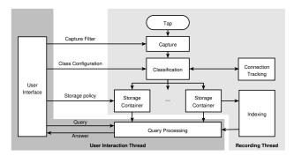
Figure 5: Time Machine System Architecture
