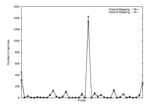
Figure 5. The distribution of AM profiles of DHCP clients for two runs separated by five months. The large spike in the graph corresponds to Windows machines not running any public services.
