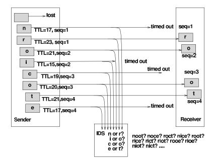
Figure 2. Evading a NIDS by manipulating the TTL field [HKP01]. The NIDS is 15 hops from the sender, but the receiver is 20 hops from the sender. Packets with an initial TTL greater than 15 but less than 20 will be seen by the NIDS but will be dropped before reaching the receiver. Since the retransmitted segments are inconsistent, the NIDS does not know the correct interpretation.
