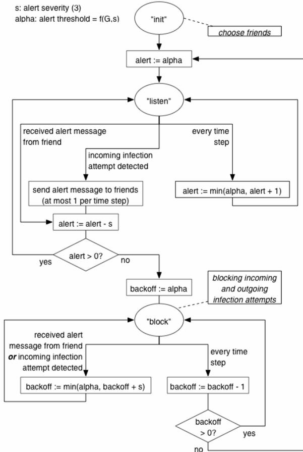
Figure 2 – Flow Diagram of Friends Algorithm
