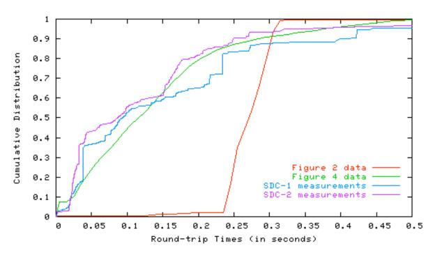
• Distributions of packet round-trip times on the congested link of two simulations, with data measured on the Internet for comparison.
