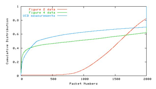
• Distributions of packet numbers on the congested link over the second half of two simulations, with data measured on the Internet for comparison.
