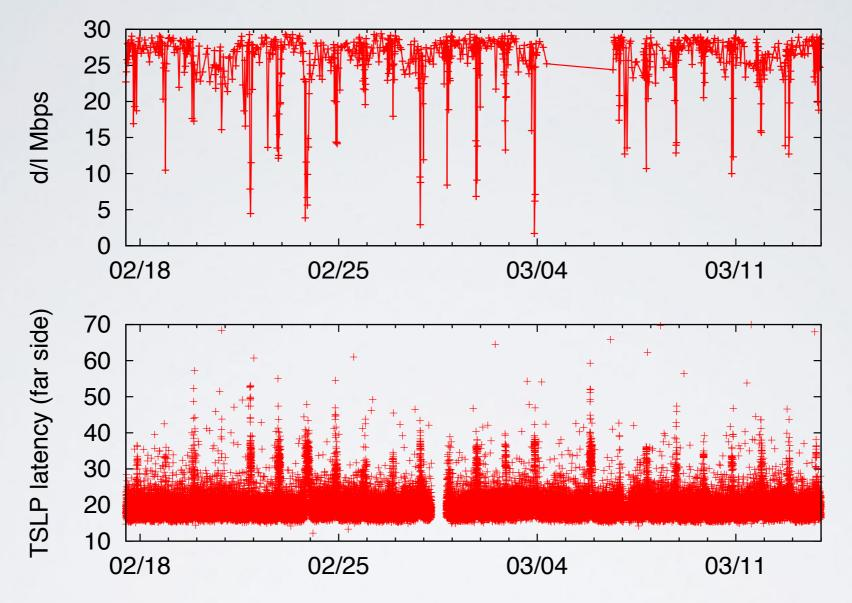
Strong correlation between throughput and TSLP latency: flows during elevated TSLP latency labeled as "externally" congested
