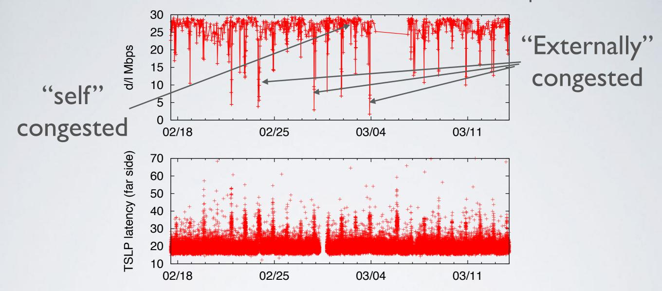
Strong correlation between throughput and TSLP latency: flows during elevated TSLP latency labeled as "externally" congested
