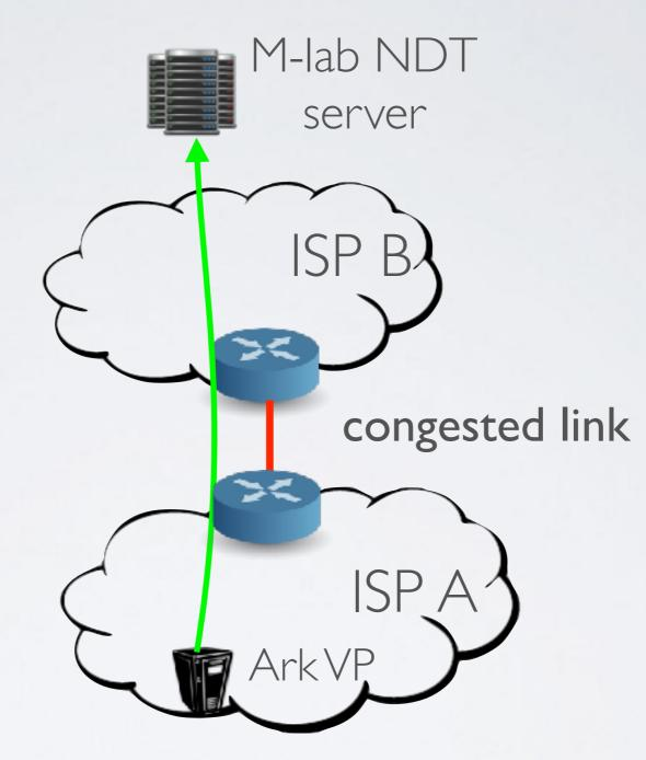
Periodic NDT tests from Ark VP to M-Lab NDT server "behind" the congested interdomain link
