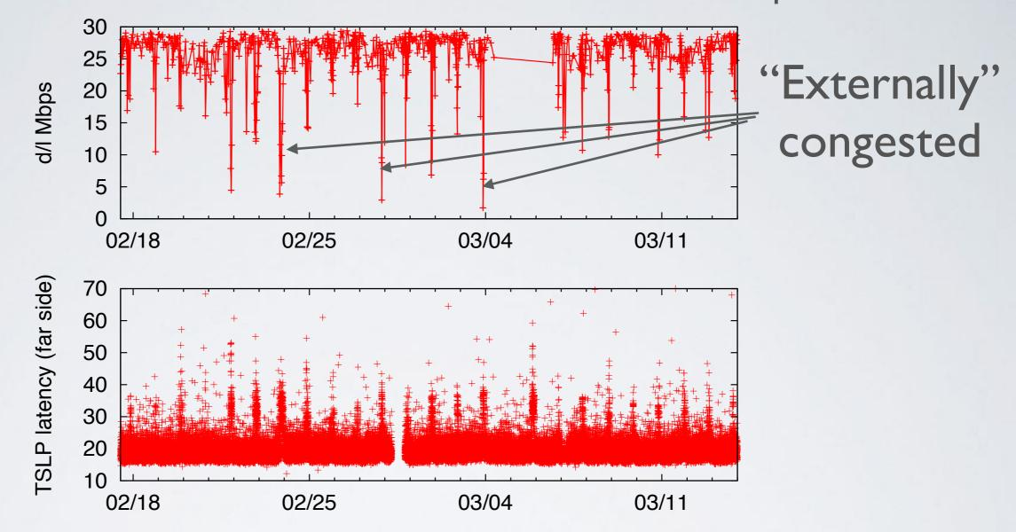
Strong correlation between throughput and TSLP latency: flows during elevated TSLP latency labeled as "externally" congested
